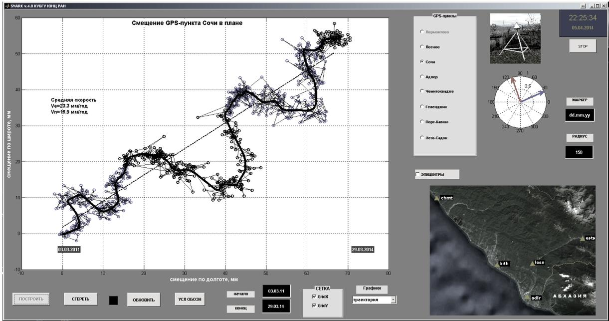
Figure 1. The slow movement of the mounting point of the GPS receiver in Sochi
