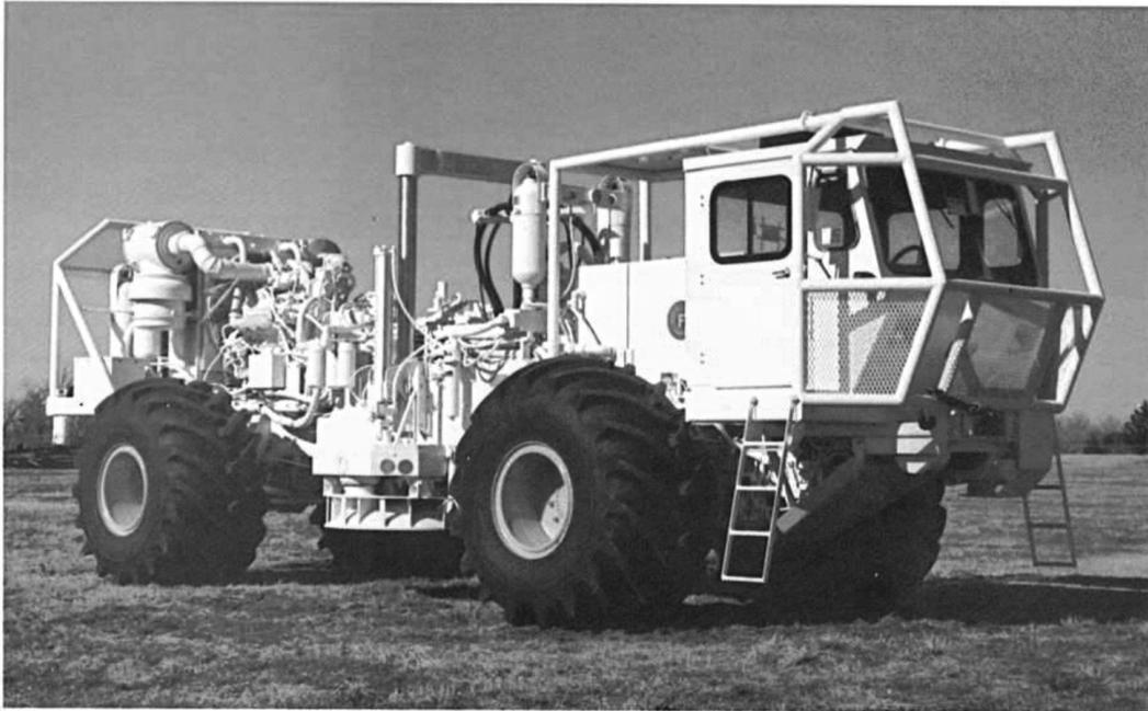
Figure 2. Vibroseis source Failing Y-3000
